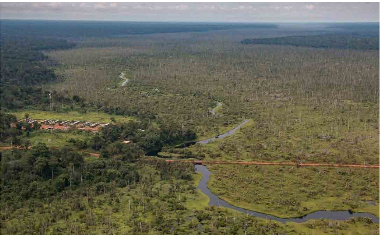
Photo taken in 2018 , at the same location, where the trees in the peat swamp are all dead, releasing carbon to the atmosphere. 7 The tree deaths are coincident with the change in drainage following the building of the road. Dieback like this has not been seen elsewhere in the region where there was no road-building.
