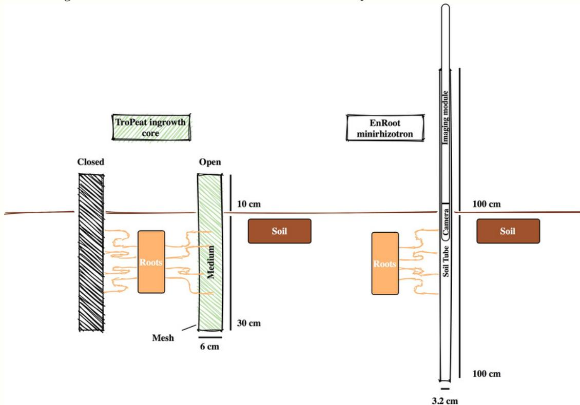
Sketch portraying the TroPeat ingrowth core and the EnRoot minirhizotron methodologies and their primary components. The medium used for the ingrowth core is homogenised peat from layers below the root mat.
